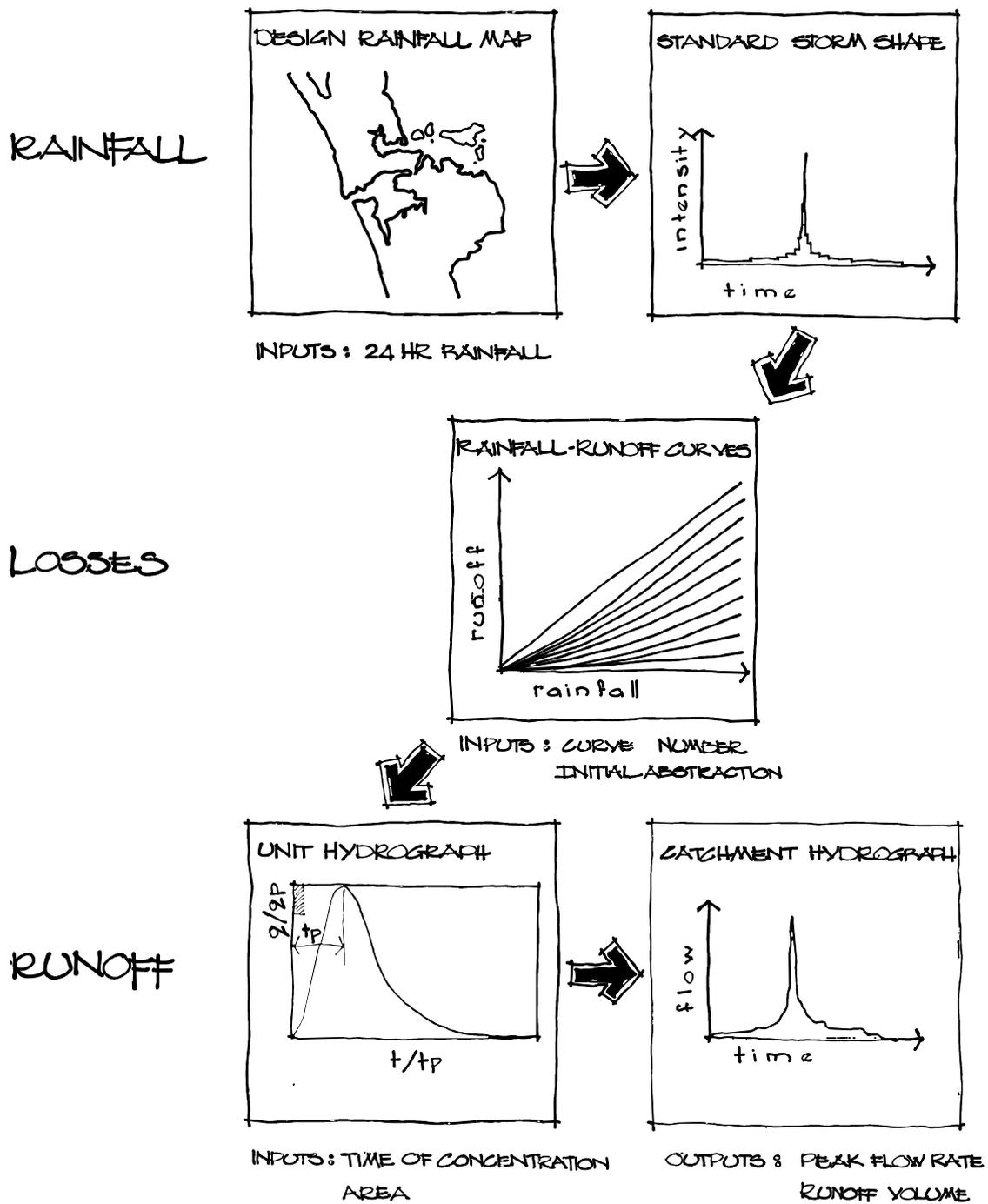
Figure 1.1 - Process diagram for the Stormwater Model
